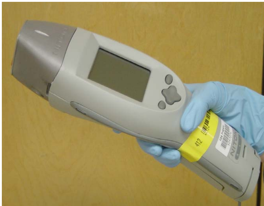
Figure 1. Photograph of Niton model Xli728 portable XRF analyzer.
